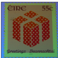
1. Visual light on edge of stamp phosphor during excitement by ultraviolet light.
